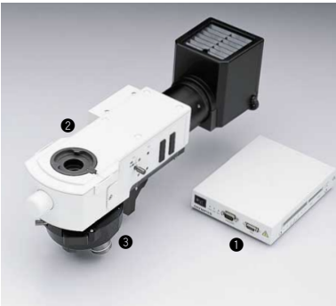
1 BX-REMCB control box for motorized nosepiece and BF/DF illuminator 2 BX-RLA2 motorized BF/DF reflected light illuminator 3 U-D5BDREMC Motorized Nomarski DIC quintuple BD revolving nosepiece
