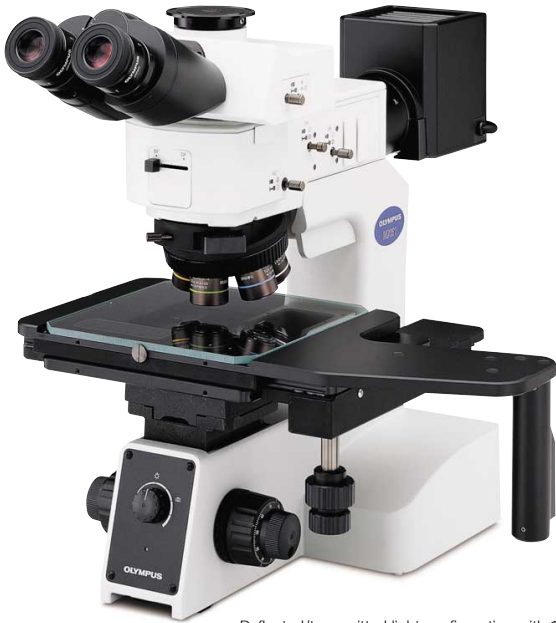
Reflected/transmitted light configuration with 150mm stage MX51+BX-RLA2+MX-SIC6R2+BH3-SPG6+MX-TILL
