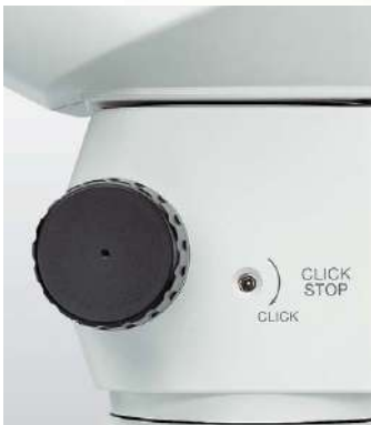
Click-stop mechanism (SZX7)
